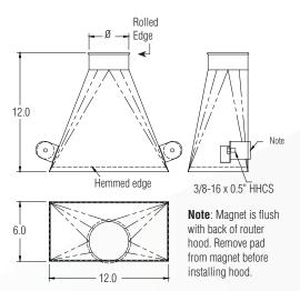
Temperature Rating: Max. temperature limited to 300°F if magnets used, due to physical characteristics of the magnets' Ferrite construction.
